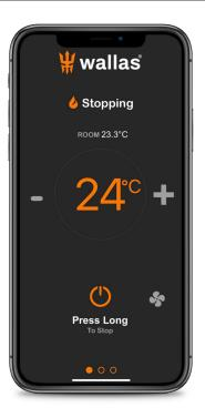
Press and hold the **Start/Stop Icon** down for 2 seconds.
