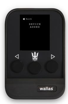
Once the pairing has been successful, it is confirmed on the control panel with DEVICE ADDED.
