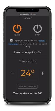
Tap on the **safety warnings** in blue to read the safety disclaimer. Follow the safety precautions to ensure all persons and property are safe prior to starting the heater. Tap on the white box to add a check mark to agree to the safety guidances.
