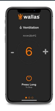
Press and hold the **Start/Stop Icon** down for 2 seconds to start the heater.
