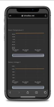
Heater requires at least 12 V to start. Check the battery voltage by scrolling down to the bottom of the page.
