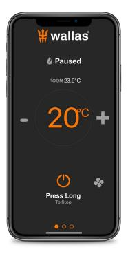
Pause Mode automatically turns the heater off if the temperature remains +2 C (3 F) above the set level for 1/2 hour due to local ambient conditions.
